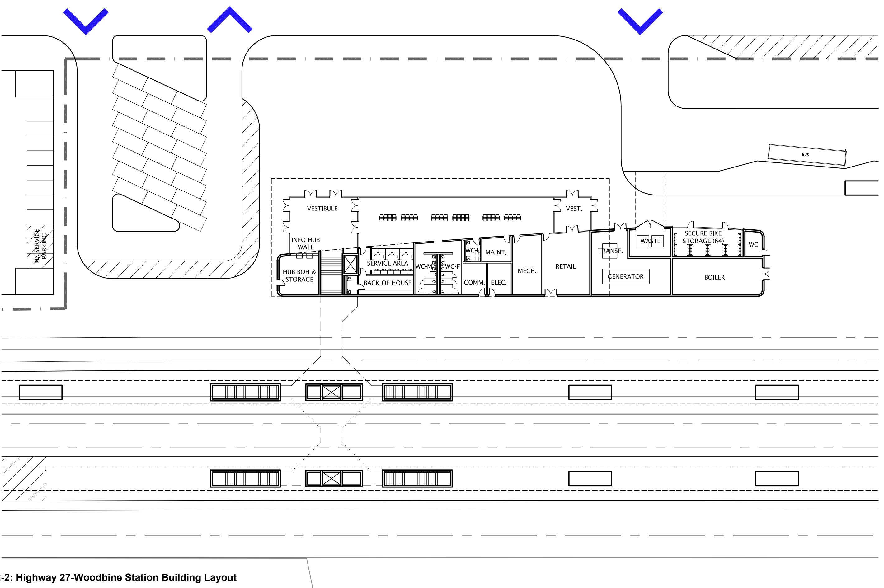
Figure 2-2: Highway 27-Woodbine Station Building Layout
